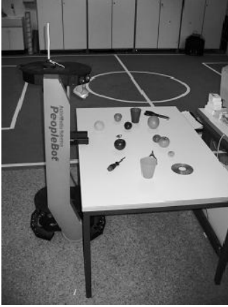
Fig. 1. Left: Robot on which the cortex model has been implemented to demonstrate a scenario involving understanding simple sentences as well as seeking and pointing to objects lying on a table. Right: Interaction of the different areas of the cortical model (v: visual, l: location, f: contour features, o: visual objects, h: haptic/proprioceptive, p: phonetics, s: syntactic, a: action/premotoric, g: goals/planning) and their rough localization in the human brain
